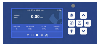
LCD Display (Real-time show the Airflow Velocity, Time, Temperature, UV life and Filter life etc.)
