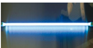
UV Lamp (Emission of 253.7 nanometers for most efficient decontamination)
